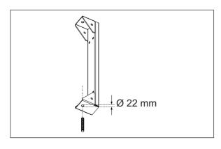
Anchor all the legs (1) to a level ground with proper anchor bolts (not included in the scope of supply). Layout as per footprint of the legs mounting kit.
