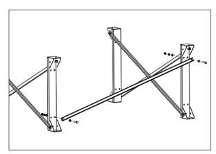
Fix the lateral wind braces (3) to the legs with the M16 screws, washers, growers and nuts.
