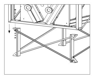
With a crane, carefully position the cooler on the legs and support the unit weight. Always follow guidelines and instructions as given in the Air Cooled Liquid Coolers Product Manual and the Alfa-V Instruction Manual to lift the unit.
