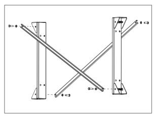
Fix the frontal wind braces (2) to the legs with the M16 screws, washers, growers and nuts.
