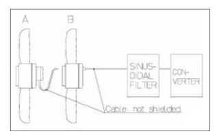
Sinusoidal filters are installed between the converter and the motor directly on the output terminals of the converter.
