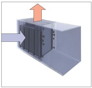
The particular design of the DCH permits the installation inside a 40' HC container. In case of running inside the container, this must be provided of 2 lateral windows in correspondence of the coils for the air inlet and 1 top window, over the fans for the air outlet.
