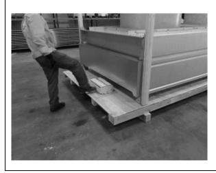
6. Open the bolts fastening the unit to package, remove fastening supports from the legs and lift the units according to **instruction manual of the unit**
