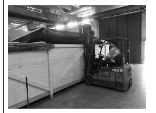
2. Open the sidewalls with crowbar, Use lifting tool to prevent wall to collapse
