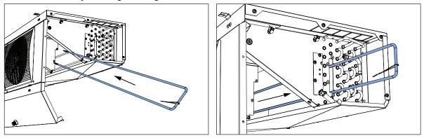
As an alternative, the heater can be inserted by the unit side only if there is adequate space to handle it.
