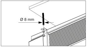
Use suitable studs when mounting the unit to the ceiling.
