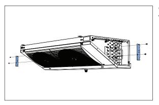
On both sides, remount the outer fixing plates with 2 self-tapping srew each.
