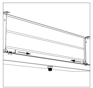
On the coil side, pull inward the spring release hinges.
