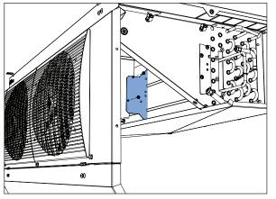
Remount the internal fixing plates, if present, by screwing the 2 self-tapping screws.
