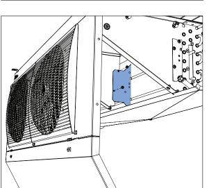
Insert the flixing clip on the heater.
