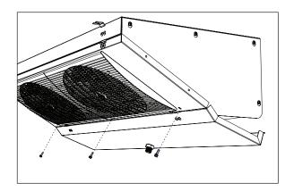
To open the fan plate, once the drip tray is unlocked, remove the screws on the fan side.
