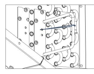
Use the fixing clip to fix the heater to the unit.
