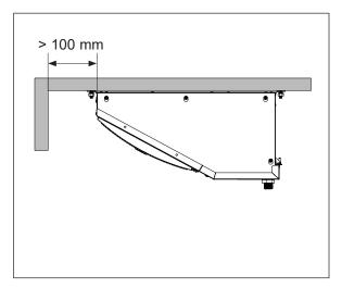
It is important to remember that the total amount of heat to be dissipated depends on receiving the full design air volume at the design entry air temperature which allows this air to be freely discharged after passing through the heat exchanger. Any restrictions may impair the performance of the cooler. If in doubt, please check with Alfa LU-VE.
