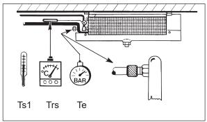
Ts1=cold room air inlet temperature. Te=evaporating temperature. It is related to the refrigerant pressure on the unit cooler outlet. Trs=refrigerant superheat temperature, on suction line near thermostatic valve bulb. (Trs-Te)=superheat
