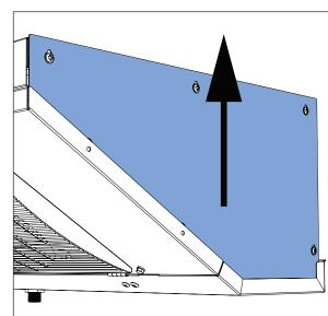
Loosen the screws and slide the panel to release it. Remove the panel.
