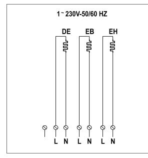
DE=electric defrost (E) EB=drip tray heater (HD) EH=heavy electric defrost (EH)
