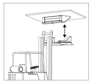
Ensure that the cooler is not lifted directly onto the drip tray or the finned coil. Utilizing the proper wooden transport beams and/or pallets prevents the cooler bending at the extremes such that the cooling circuit or other components are damaged.
